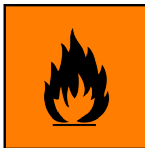
F - easily flammable
